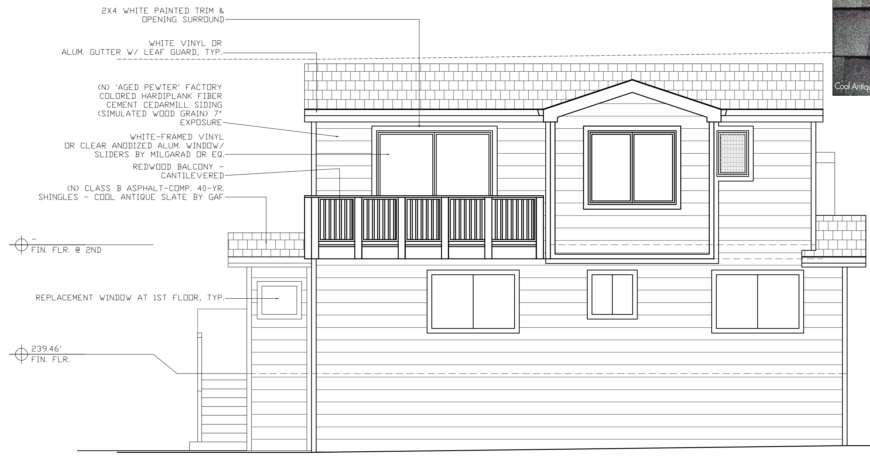
PROPOSED RIGHT SIDE ELEVATION
