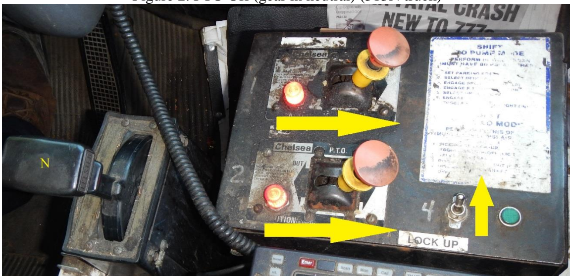
Figure 3. PTO On (gear in neutral) (513N truck)
