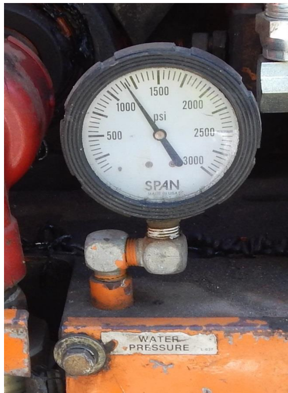
Figure 5. Water Pressure Gauge (513N truck)
