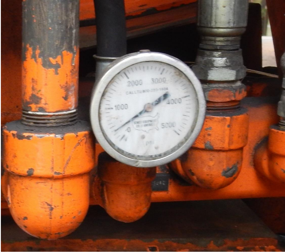
Figure 9. Water Pressure Gauge (572W truck)
