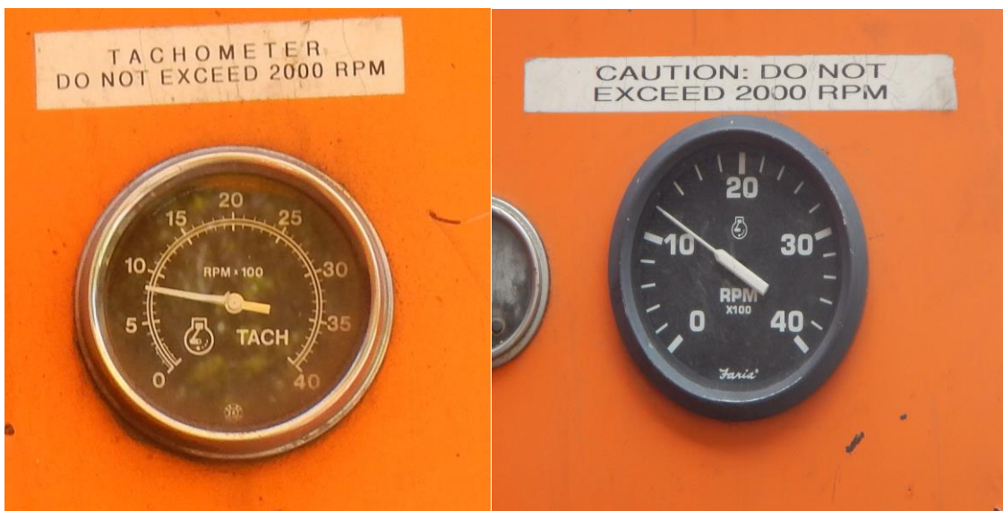
Figure 4. Typical Operating RPM for 510N Truck (Left) and 509N Truck (Right)
