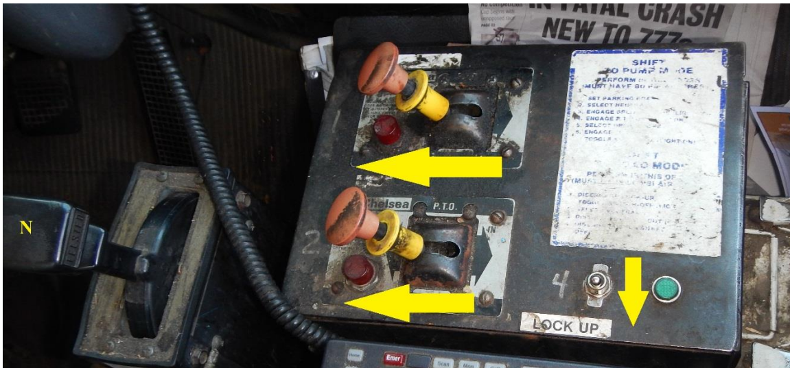
Figure 2. PTO Off (gear in neutral) (513N truck)
