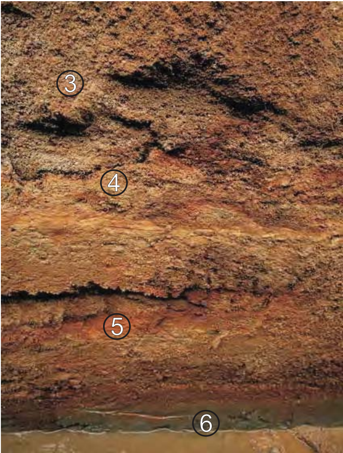
Station 0+18: Unit 3 - 6, lines not drawn so contacts are not obscured: Note thin black sand at top of Unit 4, horizontal contact between Units 5 and 6.
